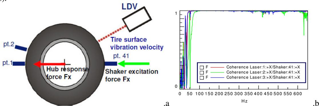
**Figure 1.** Innovative test setup for the modal characterization of a static tire<sup>4</sup>. The measurement points and the shaker excitation force location on the tire tread surface are shown for the static case. In (b) an example of coherence function for a burst chirp excitation relative to three different measurement runs.
