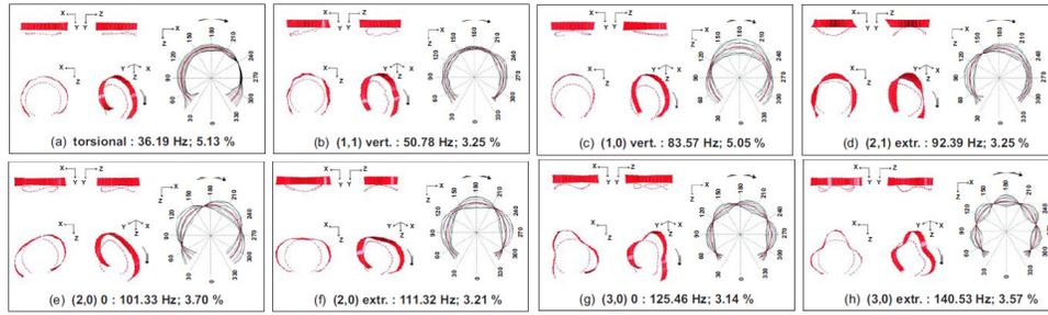
**Figure 4.** Operational modal parameters of a rolling tire<sup>12</sup> (speed 28.3 km/h, 5 mm high semicircular cleat, inflation pressure 2.2 bar). Mode shapes are shown in a fixed reference system.
