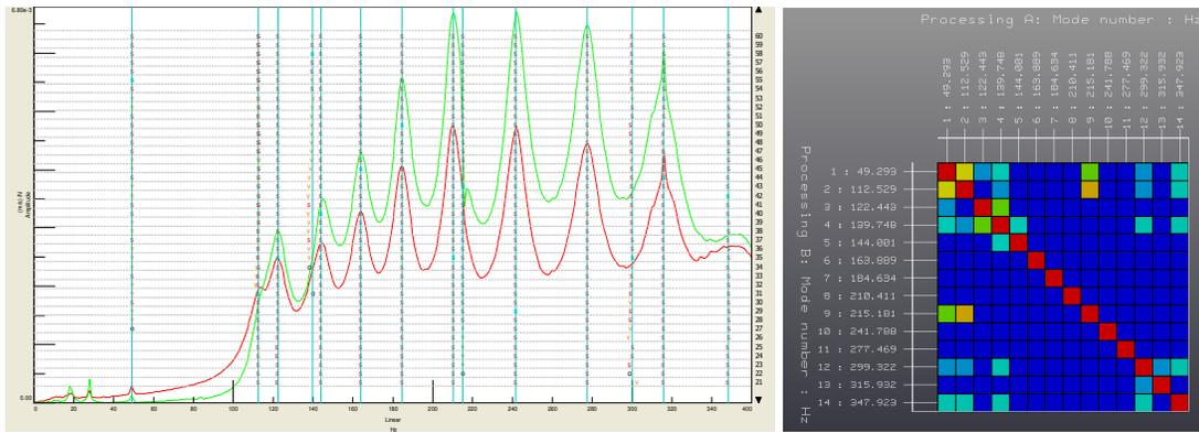
**Figure 3.** On the left, stabilization diagram relative to the unloaded tire measurements (LMS Polymax algorithm<sup>9</sup>). On the right, Modal Assurance Criterion applied to the corresponding set of modes.
