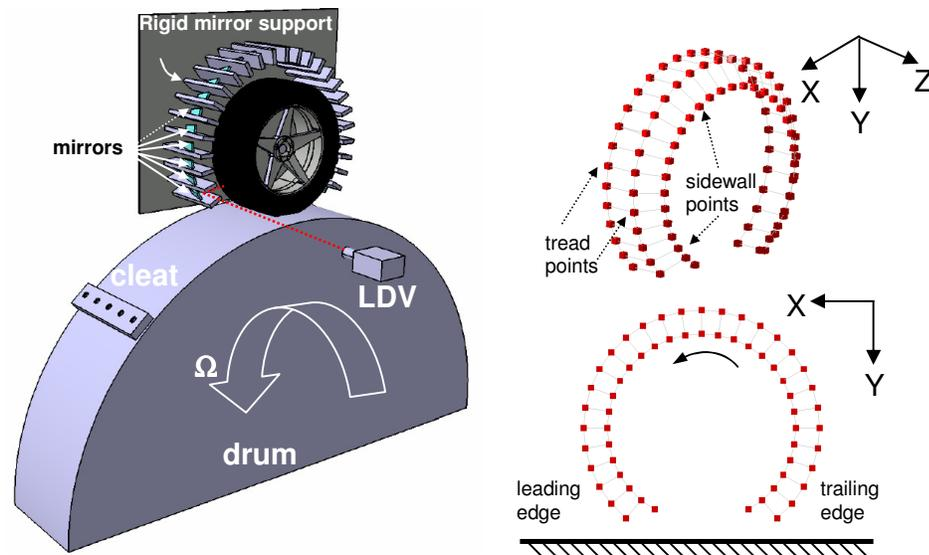
**Figure 2.** Innovative test setup for tire rolling vibration measurement by means of a Laser Doppler Vibrometer. On the right, a typical measurement grid is reported in an absolute reference system.
